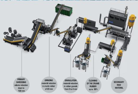
Forrec installation for the tyres recycling has a production cycle to obtain secondary raw material in different granules sizes with the simultaneous separation of steel and textile fiber.
