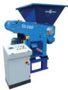
The pre-shredder is equipped with a hopper with a 4.5 ft x 3.5 ft feeding inlet. The hydraulic feeding system, via the 400 mm stroke plunger, ensures extreme ease in adjusting the pressure and speed, adapting to the various types of material to be treated.
