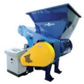
The pre-shredder is equipped with a hopper with a 5 ft x 4 ft feeding inlet. The hydraulic feeding system, via the 400 mm stroke plunger, ensures extreme ease in adjusting the pressure and speed, adapting to the various types of material to be treated.
