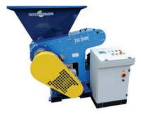
The pre-shredder is equipped with a hopper with a 4 ft x 3.5 ft feeding inlet. The hydraulic feeding system, via the 400 mm stroke plunger, ensures extreme ease in adjusting the pressure and speed, adapting to the various types of material to be treated.
