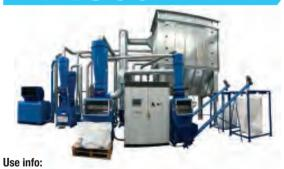
The T1500 is a plant for recycling copper or aluminium contained in electric cables separating them from the rubber or PVC sheath. Also suitable for processing rigid cables, it uses the open air circuit to control material overheating issues.
