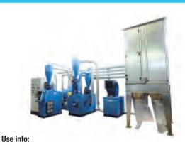
The T750 is a plant for recycling copper or aluminium contained in electric cables separating them from the rubber or PVC sheath. Also suitable for processing rigid cables, it uses the open air circuit to control material overheating issues
